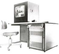
All Comtal digital image display systems work on a 512 x 512 picture matrix, coupled with a special picture tube, to produce a bright flicker-free picture with highest real-time spatial resolution. Large screen, full color presentation has a maximum resolution of 256 brightness levels for each of the three primary colors.
