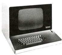
Lexicon, Inc. announces a new alphanumeric CRT display system for Nova series computers. The new display system, called Lexiscope 2000A, features high speed operation and highly flexible "intelligent interface electronics are contained terminal" capabilities through CPU on a single Nova plug-in board.
